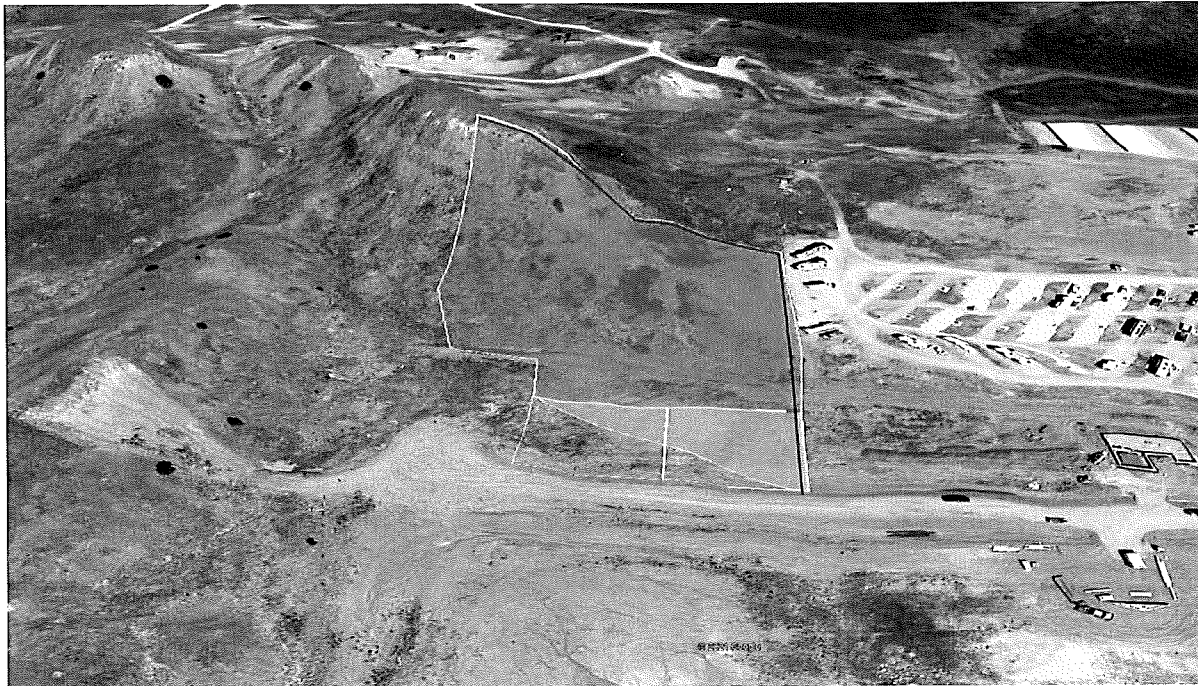
Image 3: Drainage area & longest flow path used in designing Lot 9 ditch, view North, vertical scale exaggerated for clarity.
