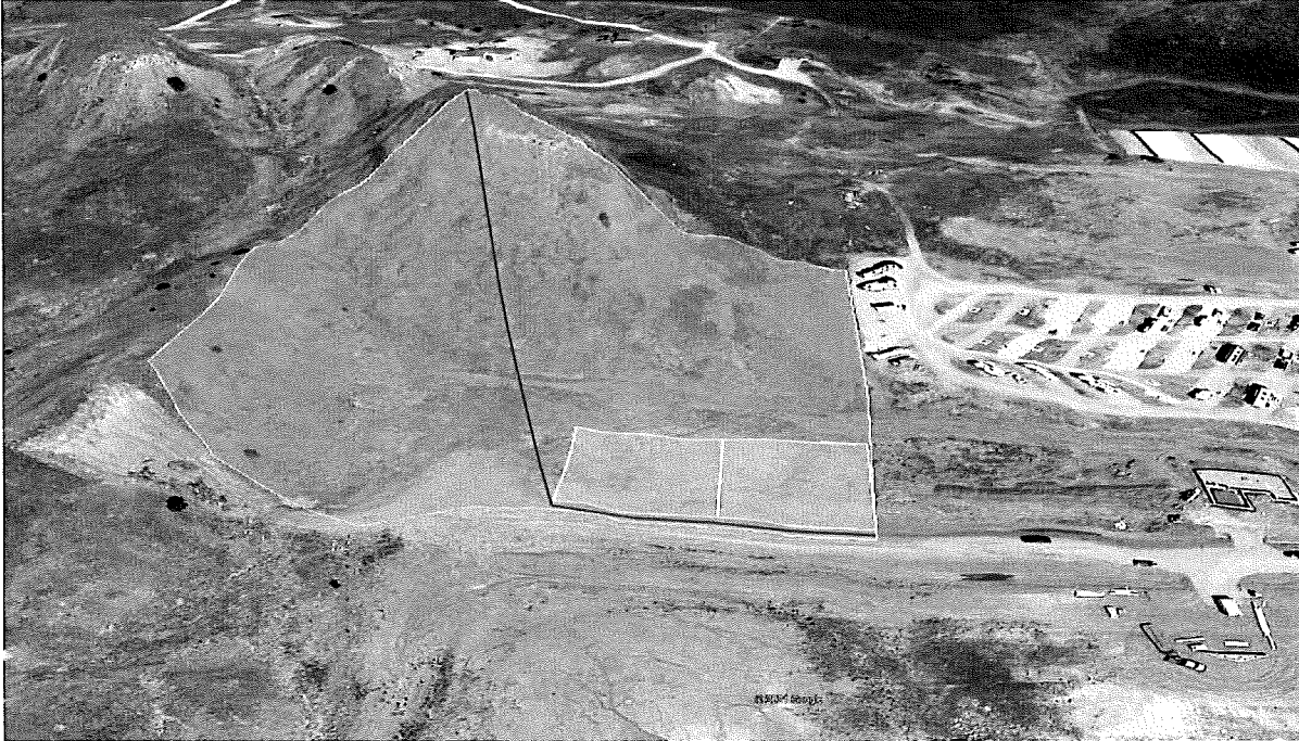
Image 2: Revised drainage area / longest flow path incorporating additional runoff from the north. View North, vertical scale exaggerated for clarity. (Google Earth)
