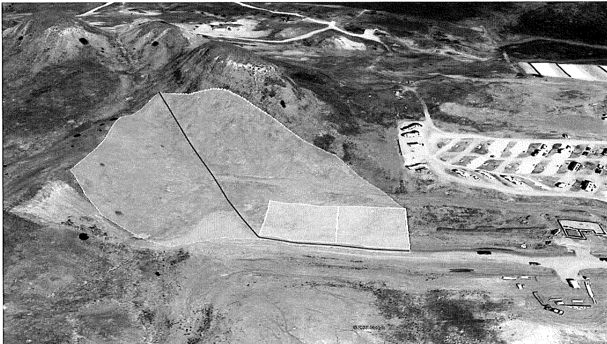
Image 1: Drainage area & longest flow path used in original 2016 design calculation. View North, vertical scale exaggerated for clarity (Google Earth)
